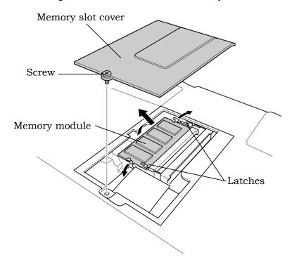
Figure 4-8 Removing the memory module
